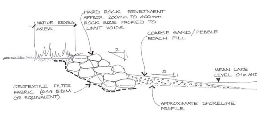
Figure 4 - Revetment for low to moderate wave action.
