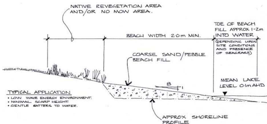
Figure 1 - Example of a Typical Beach Fill
