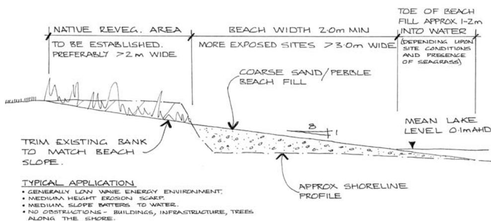
Figure 2 - Example of a Typical Beach Fill
