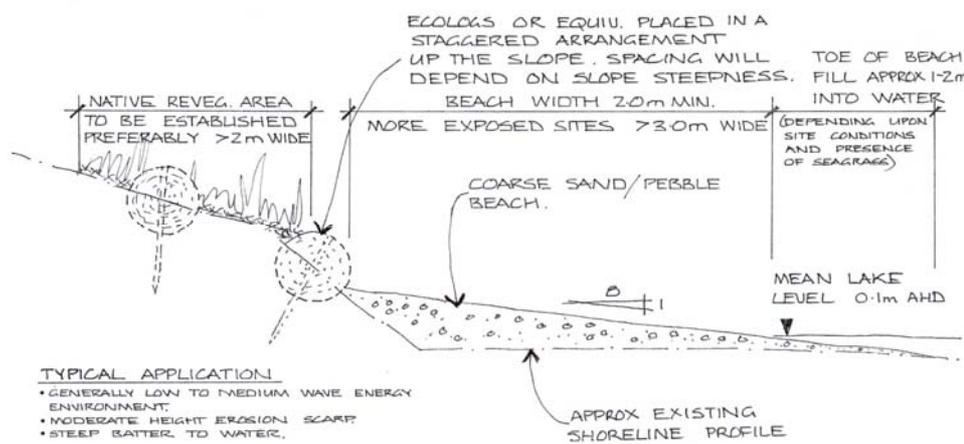
Figure 3 - Typical Beach using Coconut Fibre Log Fill
