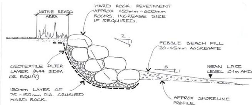
Figure 5 - Revetment for high wave action.
