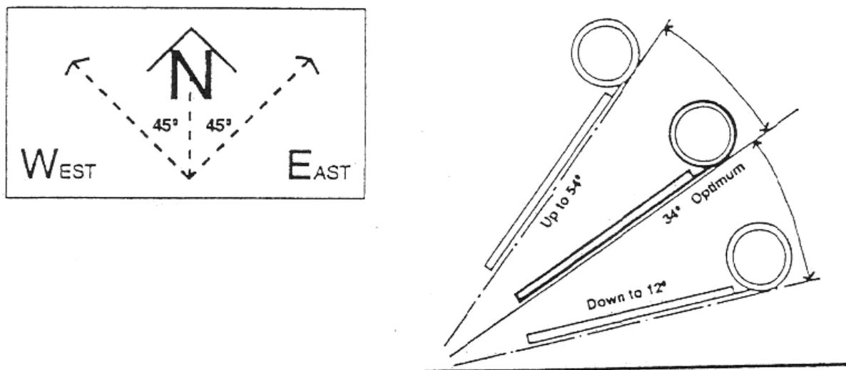
Figure 5 - Optimum range and elevation for solar collector.
