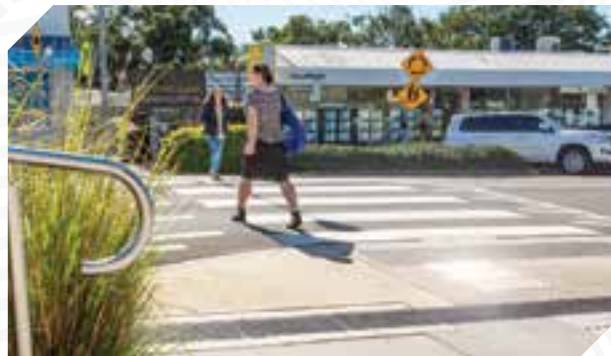
Raised pedestrian crossings to give pedestrians right of way and help manage traffic speeds
